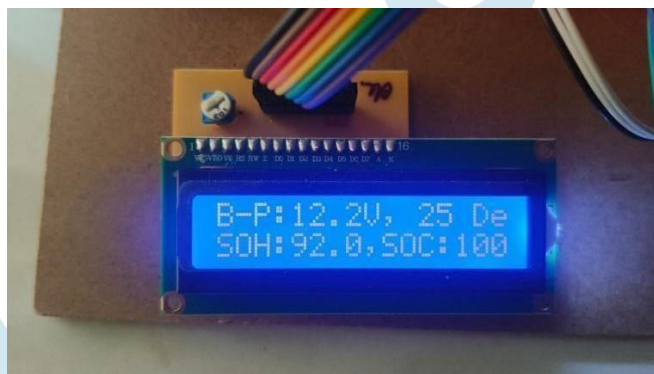
Fig 6.2 : Starting Values of SOH and SOC Displayed on LCD
