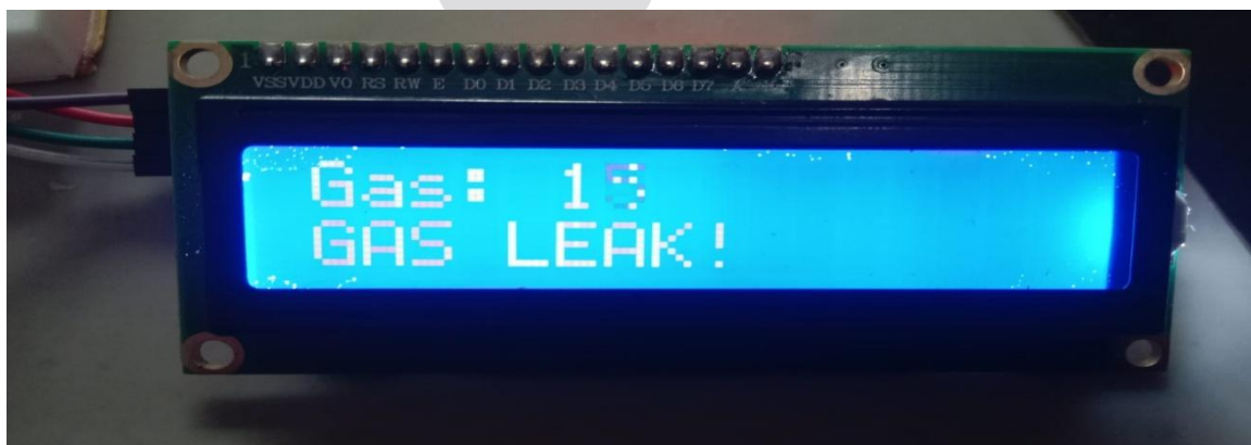
Figure : LCD Display Showing Gas Leakage Detected
