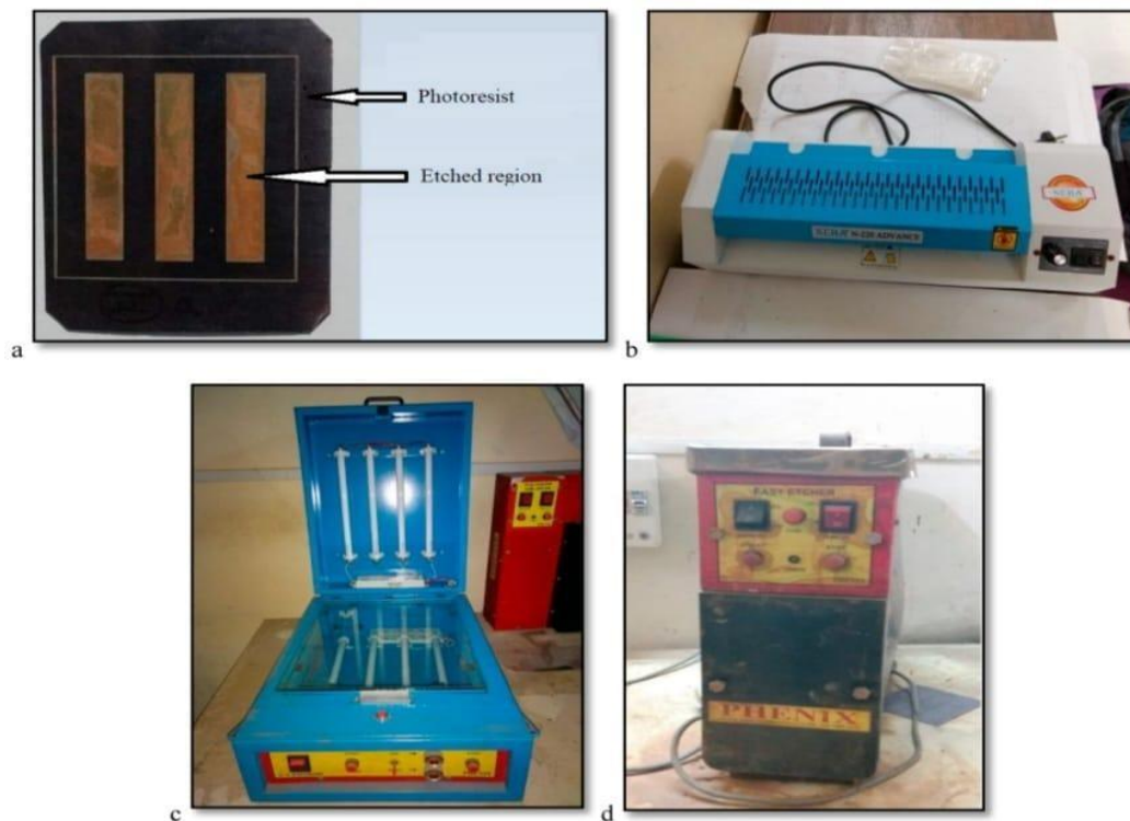
Fig 1. (a) Workpiece; (b) Lamination machine; (c) UV exposure unit;(d)Etching tank
