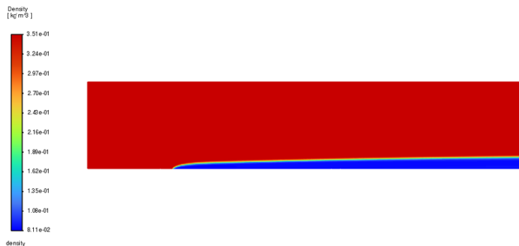
Fig. 4.3: Density Contours ( \text{kg/m}^3 )
