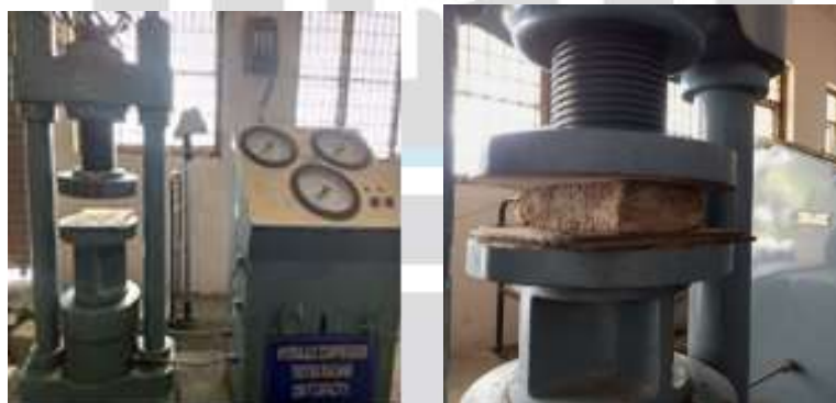
Figure.18. Hydraulic compression testing machine used for compression test.
