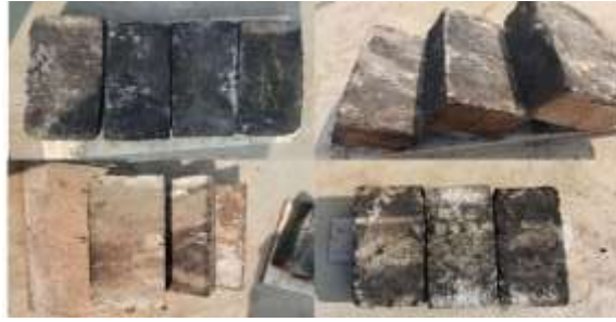
Figure.16. Drying of Waste reinforced mud bricks
