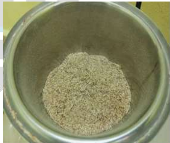
Figure.7. Grounding of rice husk into fine powder
