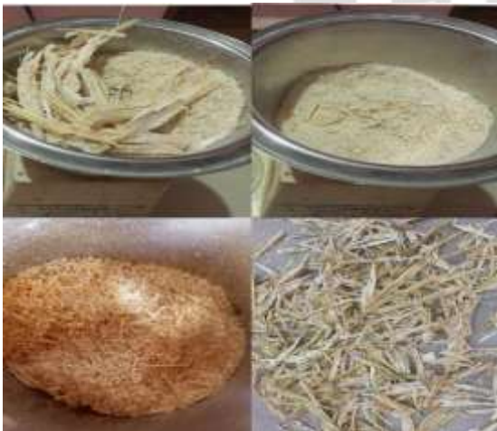
Figure. 6. Grinding of Sugar cane bagasse
