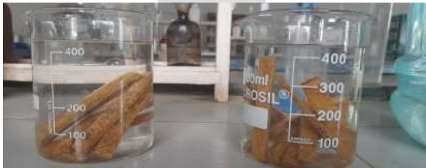
Figure 6: Immersion of fine fiber and coarse fiber in a saline water.
