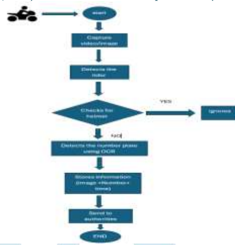
Fig:2 Flowchart for Helmet and Number plate detection
