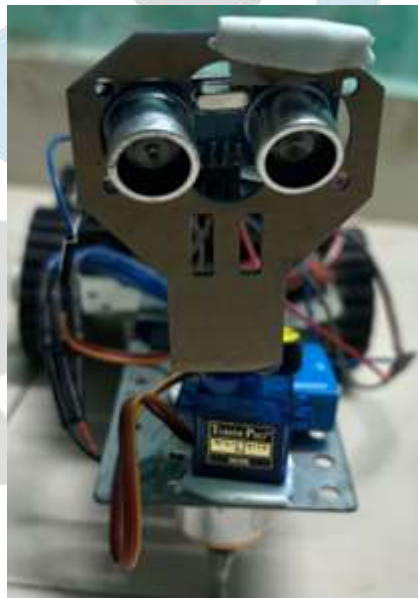
Fig. 4: Obstacle Detection Mechanism
