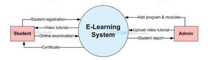
The Data Flow Diagram (DFD) provides a clear visual representation of how data moves between different components of the LMS. It illustrates interactions between users, the system's database, and various application modules, ensuring a structured understanding of the workflow.
