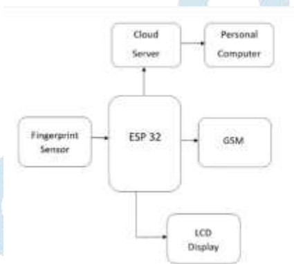
Fig 1: Block Diagram of Vote Verify
