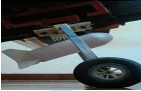
FIGURE 6. Dropping Mechanism of Electric Aircraft
