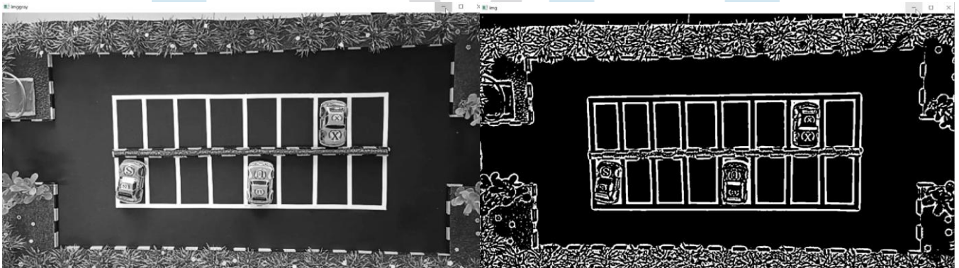
Fig 4: Conversion of frames to calculate pixel count
