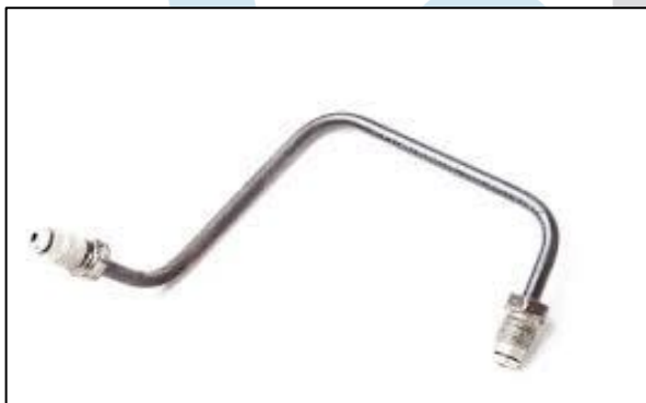
Fig 7: Image of a commercially used Brake line
