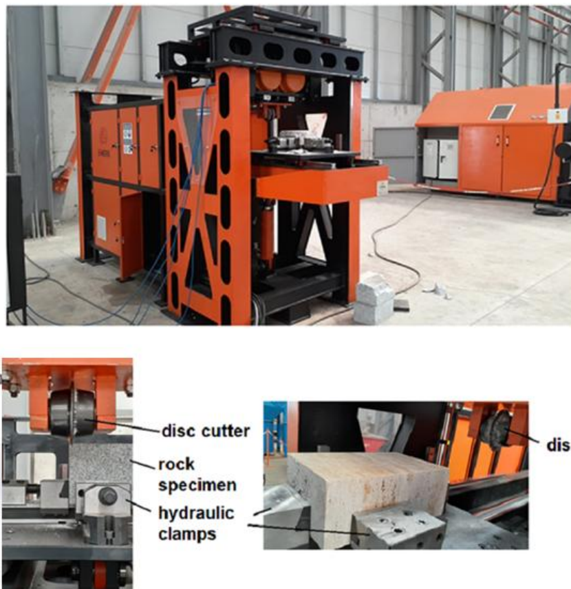
Fig.4. General view of the DCD technology prototype and a single oscillating disc cutter
