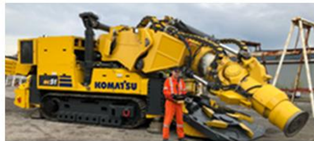
Fig. 3. Hard rock cutters developed in recent years (a) TBM (b) mini discs Sandvik Tamrock ARM 1100, (c) ODC (left) and Komatsu MC51 (right)
