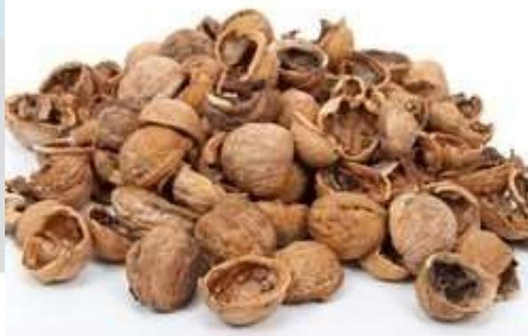
Walnut shells are a versatile abrasive media widely used in blasting, tumbling, cleaning, polishing, filtration, cosmetics, as well as non-skid applications and filler applications. Walnut shells are crushed, ground and classified to standard mesh sizes that range from coarse to fine powders.
