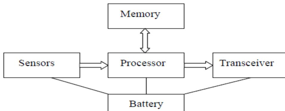
**Figure 1:- Configuration of a Sensor Node**
