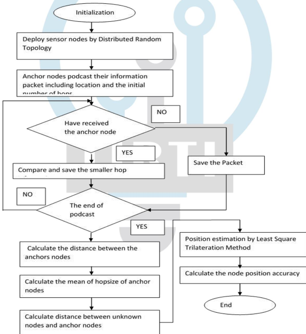
**Figure 2:- Flow-chart diagram of proposed algorithm**
