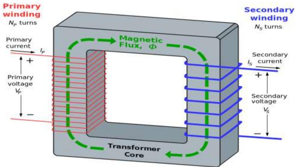
Fig. 3.3 Transformer Internal circuit
