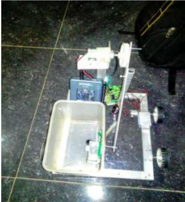
**Fig.4:** Prototype of seeds plantation robot using Lab VIEW
