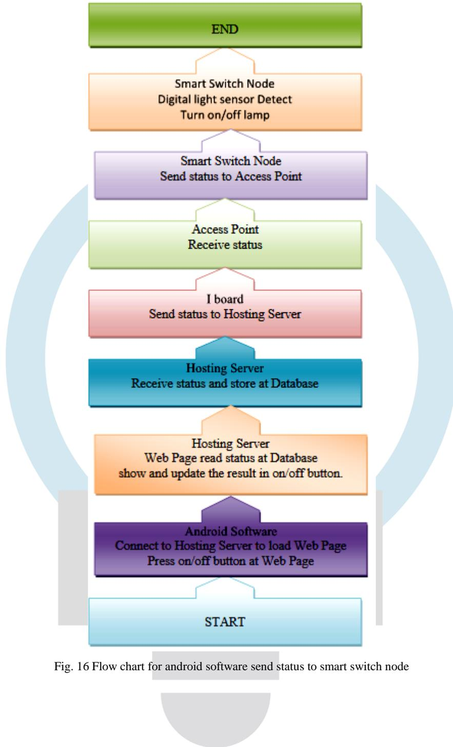
Fig. 16 Flow chart for android software send status to smart switch node
