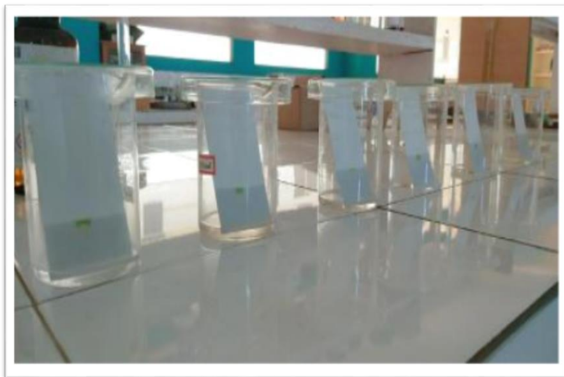
Fig No. 1 Performing the TLC of different solvent extractions. (9)
