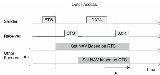
**Fig. (B) Collision and Overhearing avoidance scheme**
