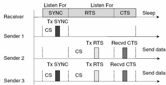
**Fig. (b) Timing relationship between a receiver and senders**
