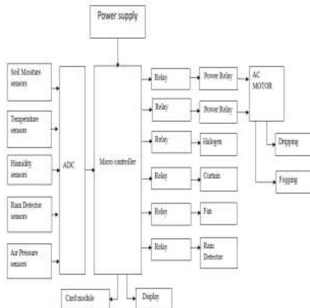
1. Sensors: we are going to use soil moisture sensors, humidity sensors, rain detectors sensors temperature sensor and air pressure sensor to sense soil moisture, humidity rain detect, temperature and air pressure respectively. These sensors sense the parameters and gives corresponding voltage output
