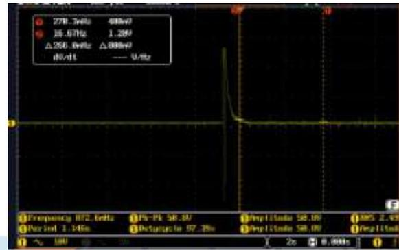
Fig. 18. Load Voltage with protection
