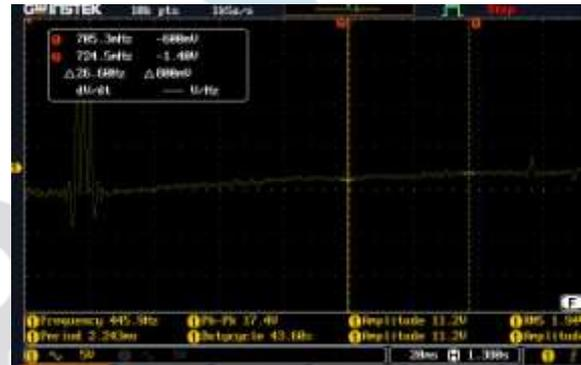
Fig. 19. IGBT collector-emitter voltage  $V_{CE}$  with protection
