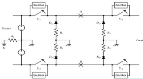
3.Implementation of the proposed protection scheme. Arrows denote the switching action when a fault is detected.
