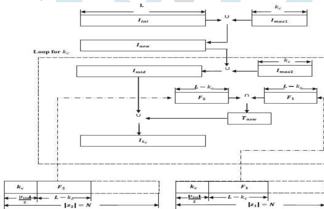
Fig.4: Description of reconstruction procedures used in MSMP method
