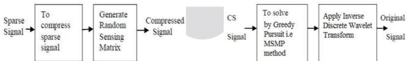
Fig.1: CS Transmitter
