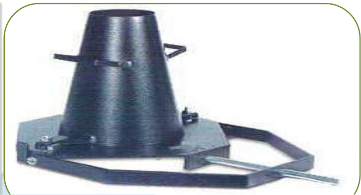
Figure 3: Concrete Flow under Slump Test and Typical Slump Cone Test Apparatus
